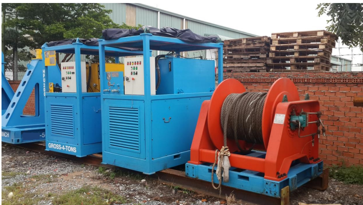
Image of hydraulic winch with HPU
